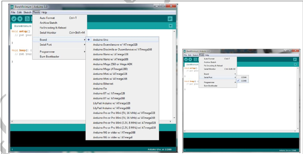
Figure 1.9: Selection of the Board and Com port.
