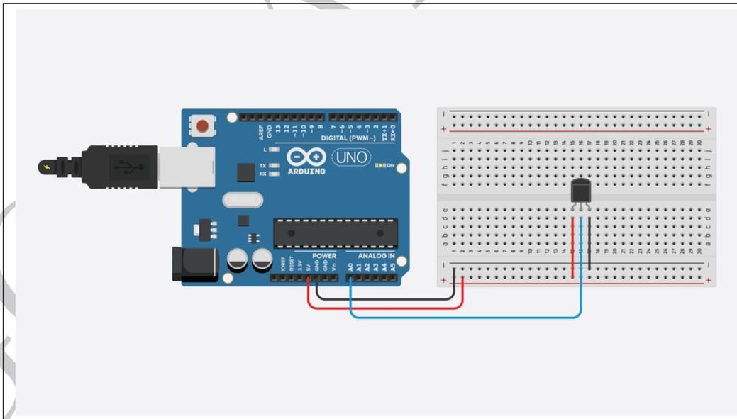
Figure 1.17: Connecting the LM 35 to the Arduino.
