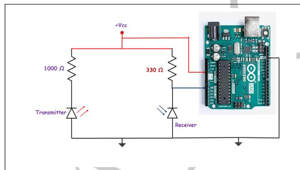
Figure 1.40: IR Transmitter & Receiver coupled to Arduino.
