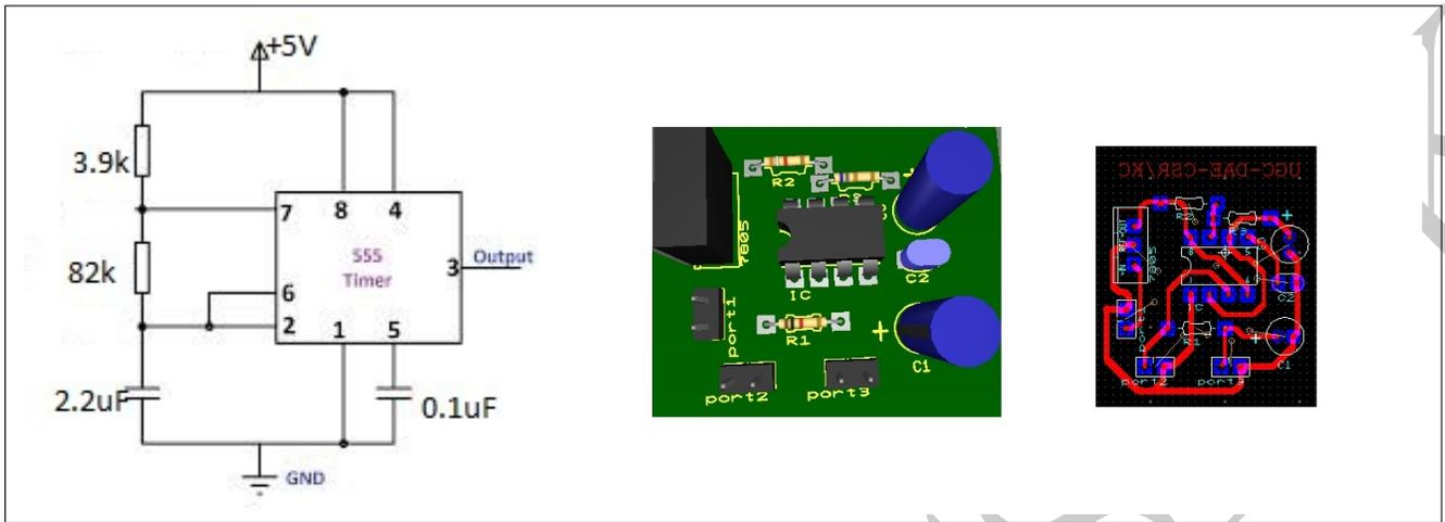
Figure 1.31: Circuit Diagram for 555 timer as Astable Multivibrator.
