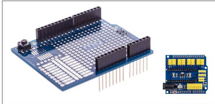
Figure 1.6: Prototype expansion boards for Arduino Uno, and Nano .
