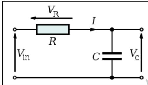
Figure 1.25: Series  $RC$  circuit.
