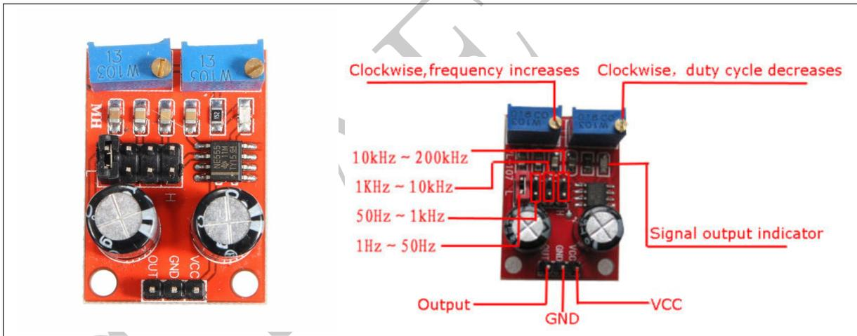
Figure 1.32: Open source 555 timer board.
