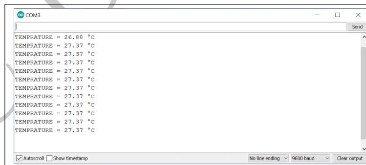
Figure 1.18: Display of the Temperature on the Serial Monitor.
