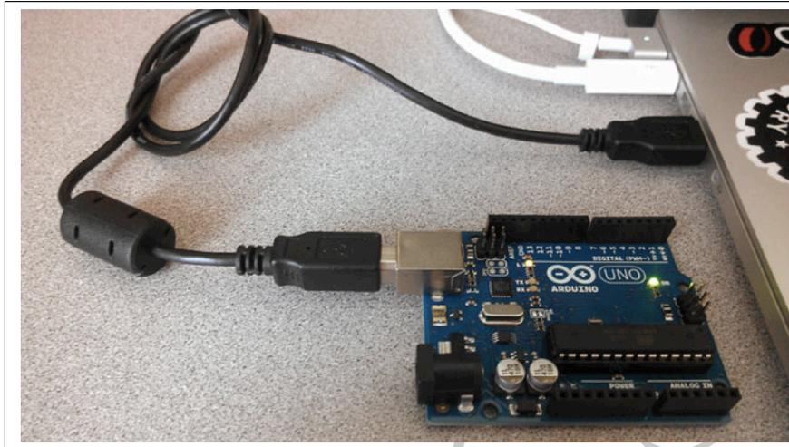
Figure 1.8: Connect the Arduino to the host computer.
