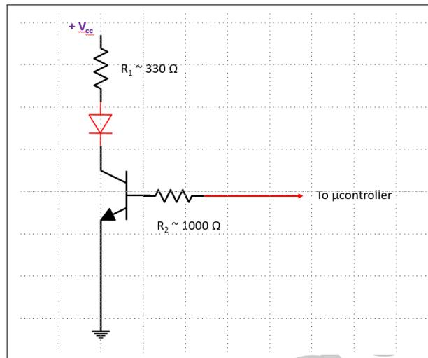
Figure 1.37: Transistor as a switch.
