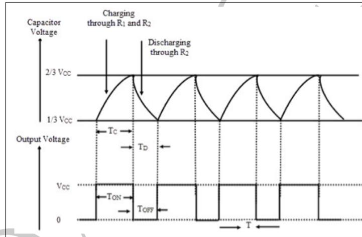
Figure 1.30: Waveforms for 555 timer as Astable Multivibrator.
