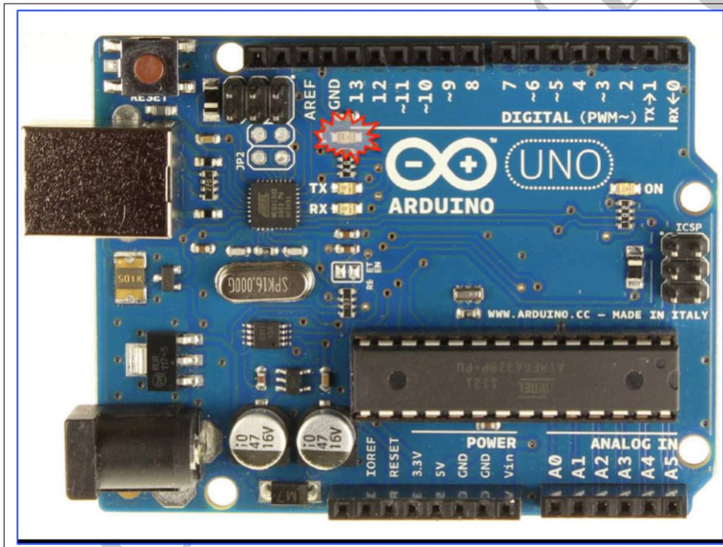
Figure 1.12: Blinking the on-board LED.
