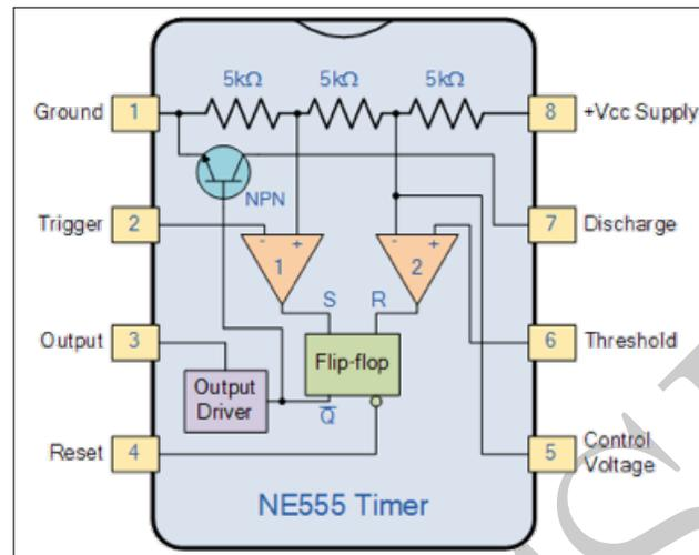
Figure 1.29: A simplified *block diagram* illustrating the internal functional blocks of the 555 timer.
