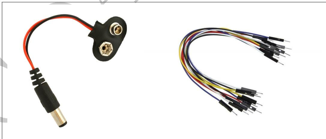
Figure 1.5: 9V snap connector and Single strand connectors .
