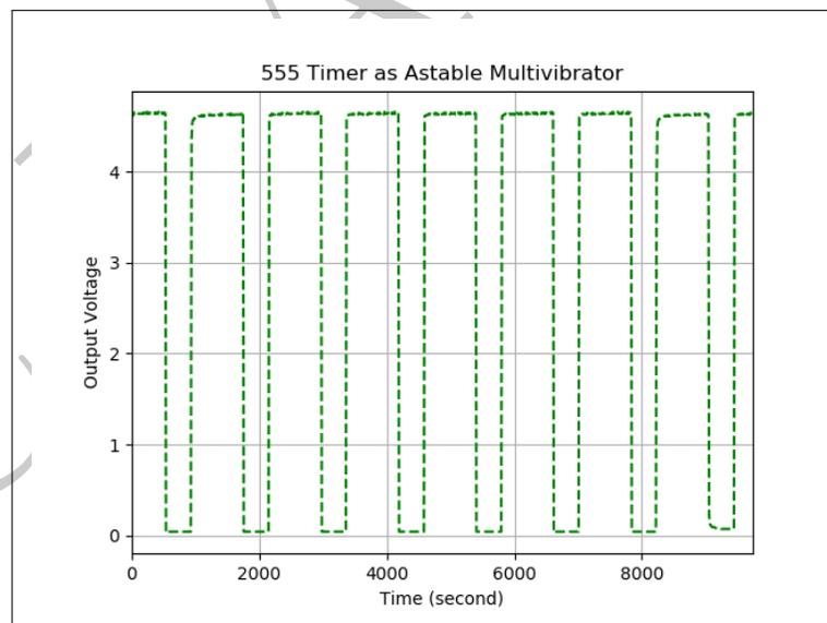
Figure 1.34: Square wave from the 555 timer board.
