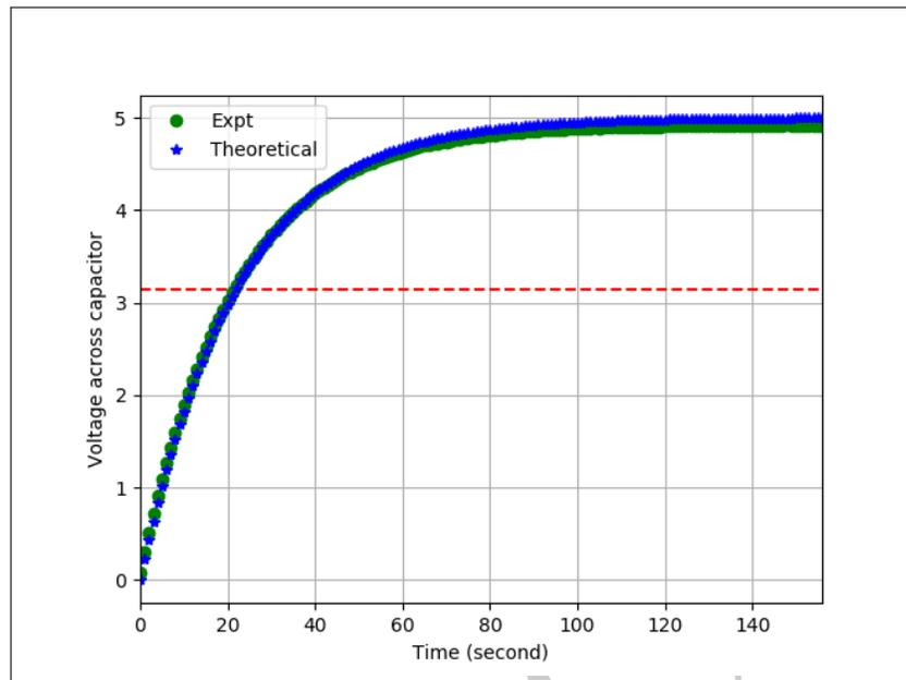
Figure 1.27: Voltage across the capacitor during charging.
