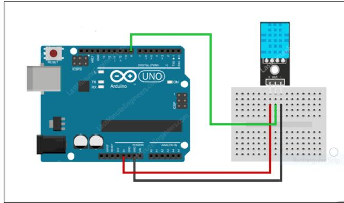
Figure 1.20: Connecting the DHT11 module to the Arduino.
