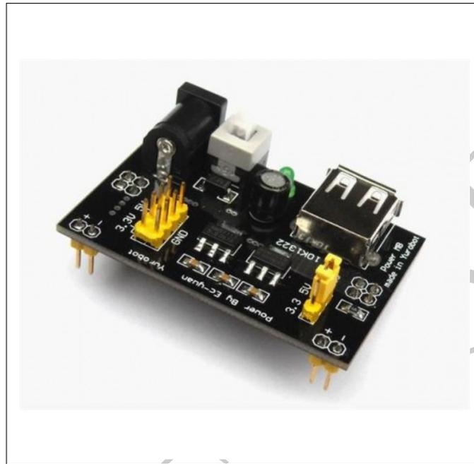
Figure 1.4: Breadboard power supply .
