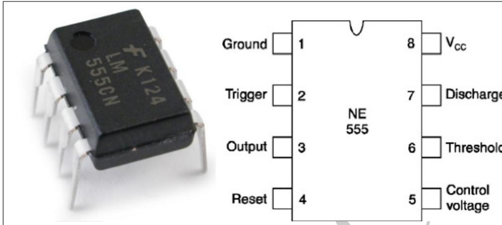
Figure 1.28: The pin configuration of the 555 timer IC.
