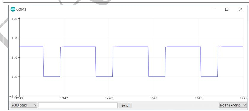
Figure 1.33: Square wave output from 555 timer.
