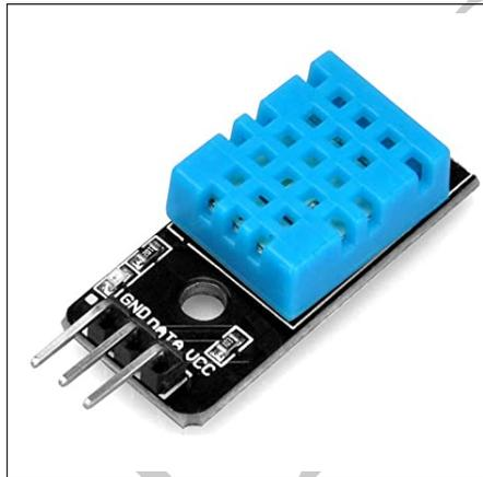
Figure 1.19: Pin configuration of the DHT11 module (The configuration is vendor dependent.)
