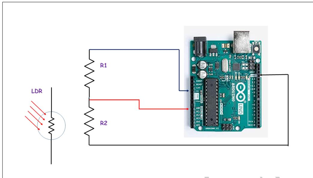
Figure 1.43: LDR connected in a voltage divider (replacing  $R_2$ ) and coupled to an Arduino.
