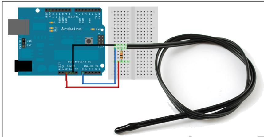
Figure 1.23: Circuit for connecting the thermistor to the Arduino.
